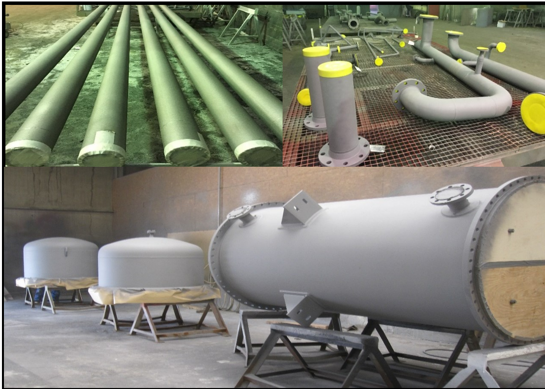
Figure 1: TGPS CUI mitigation coating - shop application prior to transport and installation.
