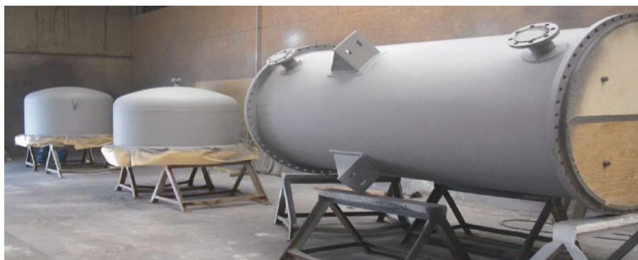
A third-generation polysiloxane coating is shop-applied to equipment prior to transport and installation. Photo courtesy of James Reynolds and Peter Bock.
